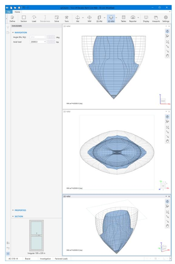
Figure 18 – Core Wall 3D Failure Surface with a Horizontal Plane Cut at P = 20,000 kip (spColumn)
