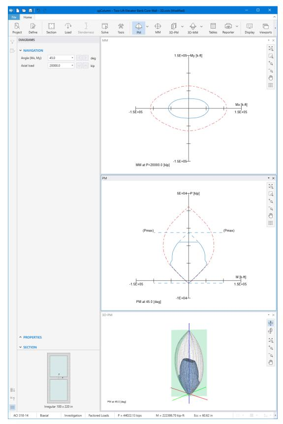
Figure 17 - Core Wall Interaction Diagram and 3D failure Surface Viewer (spColumn)
