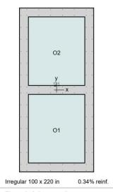
Figure 1: Column section
