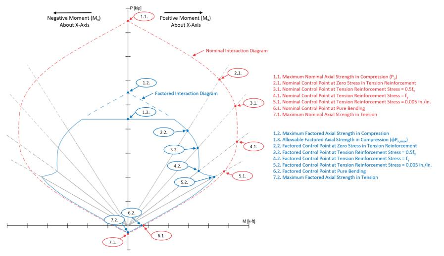
Figure 3 - Core Wall Section Interaction Diagram Control Points
