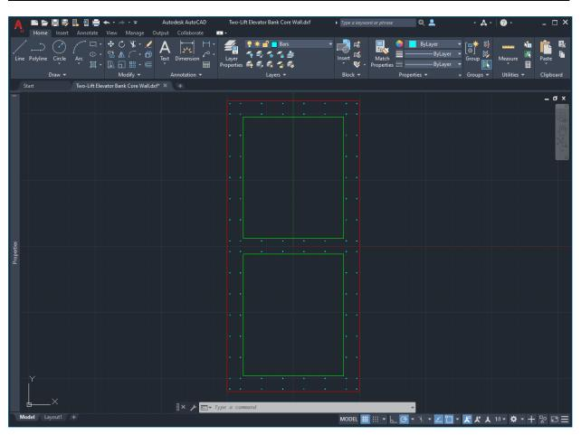
Figure 11 - Core wall Section Using AutoCad (.dxf file)
