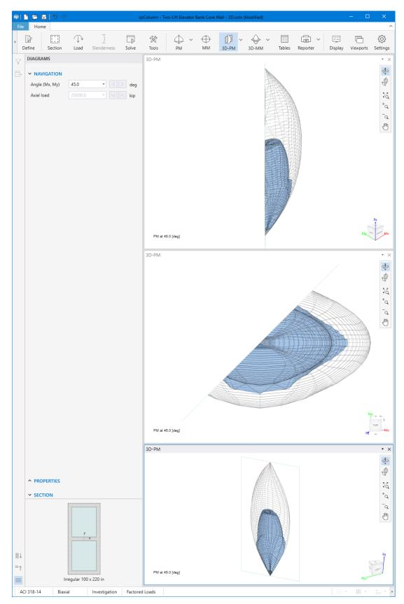
Figure 19 - Core Wall 3D Failure Surface with a Vertical Plane Cut at 45° (spColumn)
